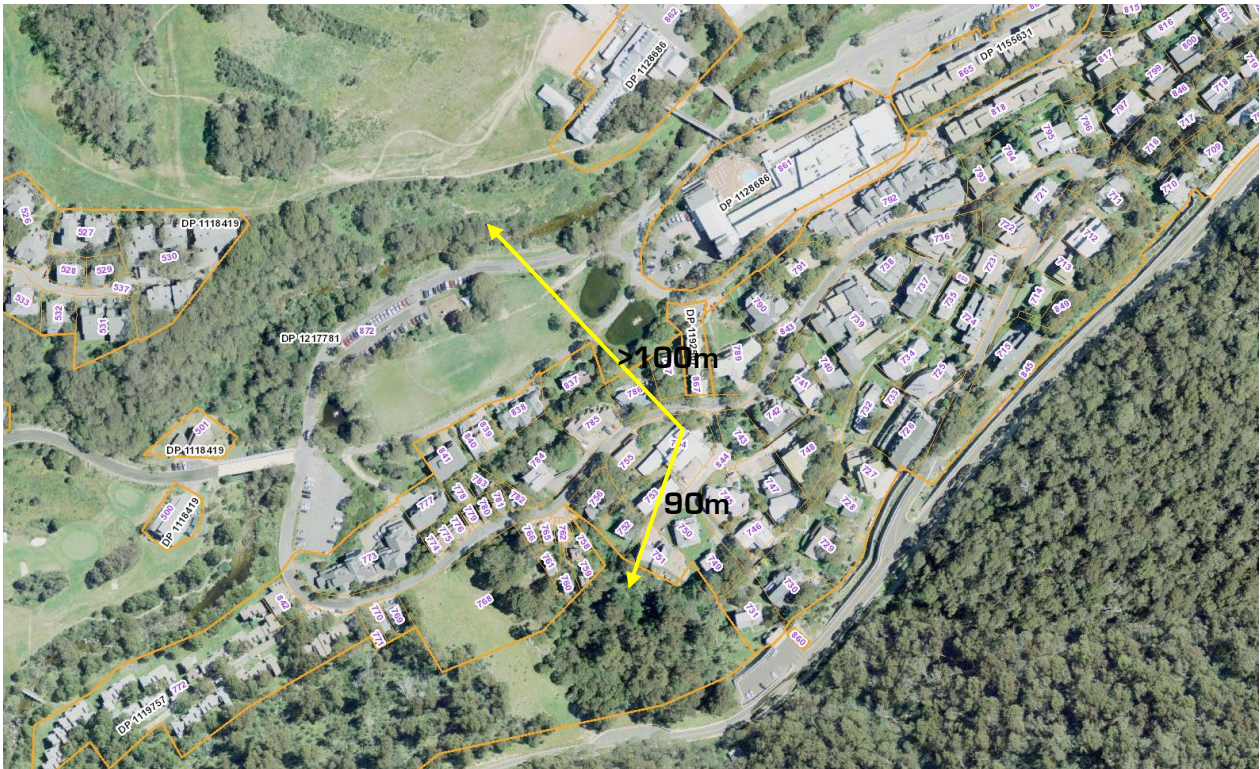
Figure 13: Aerial view demonstrating the distance to other vegetation that would have the most influence in the event of a bushfire
